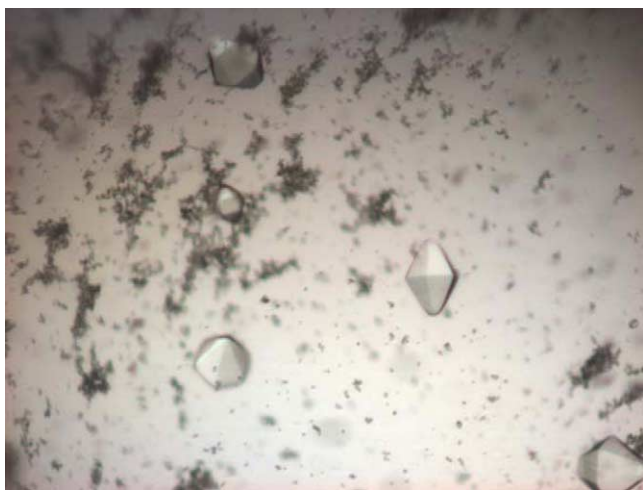
Fig. 4. Crystals of zVDR- 1\alpha,25(\text{OH})_2\text{D}_3 . The crystals were obtained in Bis-Tris 0.1 M pH 6.5, lithium sulfate 1.6 M and magnesium sulfate 50 mM. The size of the largest crystals were 200 \mu\text{m} \times 100 \mu\text{m} \times 100 \mu\text{m} .
